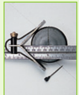
CENTRE HEAD For locating centre lines on cylindrical items.
