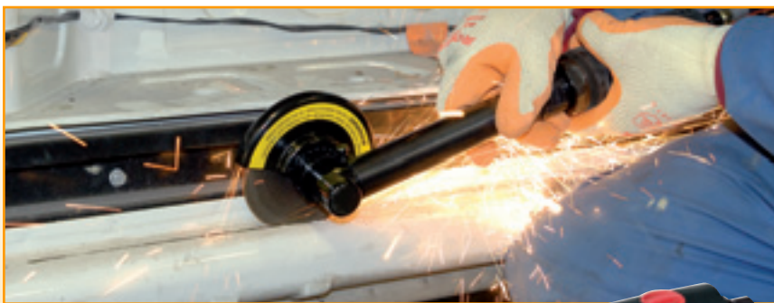
5 5220PRO 6mm Compact Soft Grip Air Angle Die Grinder with 115° head
